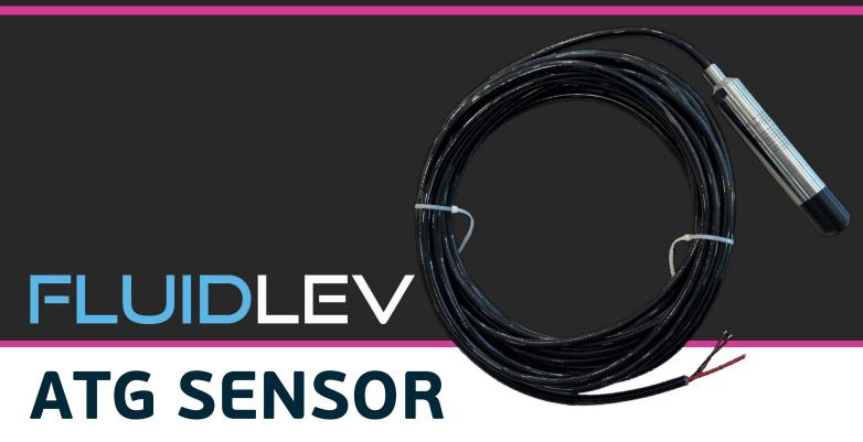
Fluidlink ATG Sensor IECEx Certified, 4-20mA, 0-3000/6000mm Range, 10m cable IECEx-certified drop-in tank sensor for hazardous fuels, including petrol and aviation. Built from 316 stainless steel with a 0-3000mm and 0-6000mm depth range and 10m high-resistance cable. Includes 25mm BSP gland for sealed installs. Compatible with Fluidlink controllers and Clarity software for full remote monitoring.
